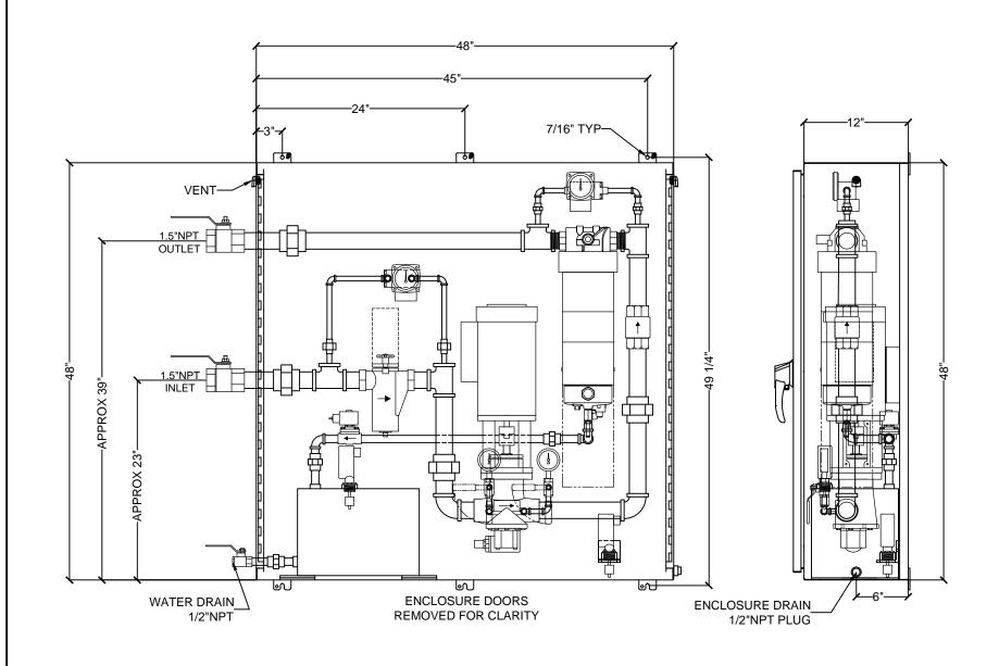
FMEZ1220 FUEL MAINTENANCE SYSTEM With GHCF COALESCER & DP SWITCH With SIMPLEX STRAINER & DP SWITCH With AUTOWATER With LEAK SWITCH NEMA 12 ENCLOSURE 48"x48"x12"
