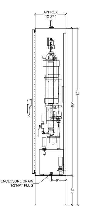
FMEZ0760 FUEL MAINTENANCE SYSTEM With COALESCER & DP SWITCH With SIMPLEX STRAINER & DP SWITCH WITH PREFILTER & DP SWITCH With AUTOWATER With LEAK SWITCH NEMA 4 ENCLOSURE 60"x60"x12"
