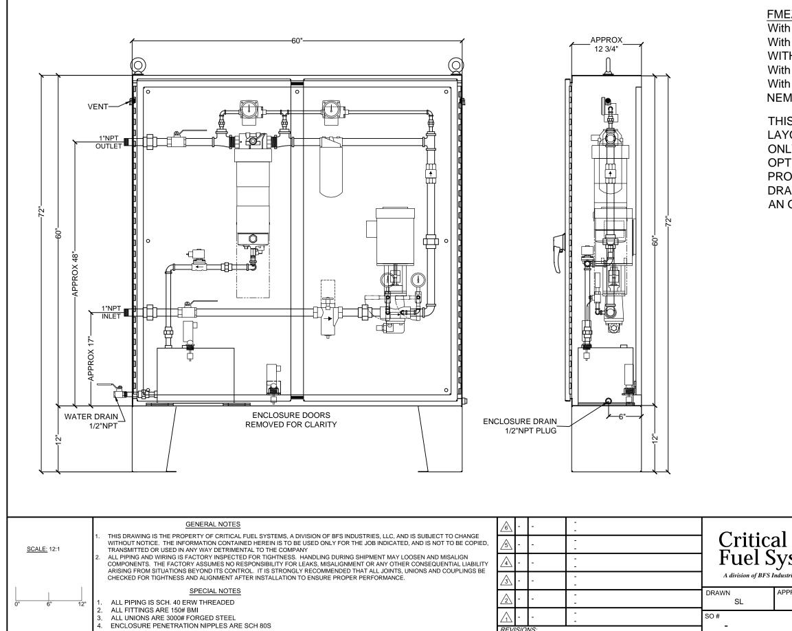
FMEZ0610 FUEL MAINTENANCE SYSTEM With GHCF COALESCER & DP SWITCH With SIMPLEX STRAINER & DP SWITCH WITH PREFILTER & DP SWITCH With AUTOWATER With LEAK SWITCH NEMA 4 ENCLOSURE 60"X60"X12"
