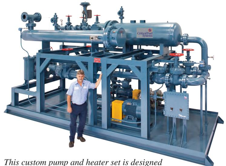
*This custom pump and heater set is designed for a flow of 10,000gph of #6 oil with a steam turbine driven pump.*
